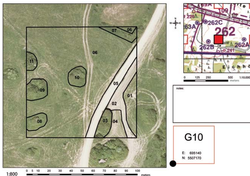
Figure 2-6: Example of a surveyed plot (G10) after subdividing the 1 hectare plot (black square) into eleven patches (numbers). Grid: UTM WGS84 Zone 32 North.
