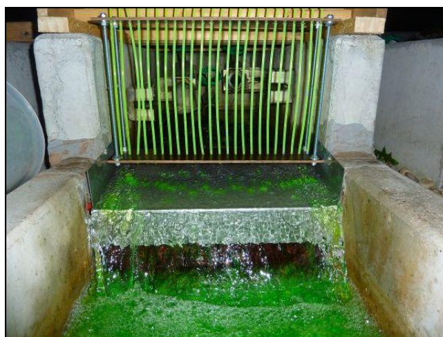
Figure A2-1 Photograph of a tracer application conducted during darkness in a vegetated stream mesocosm.
