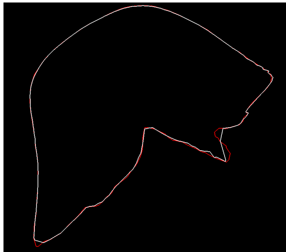
Figure 46: A problem of landmark-based shape representation is shown. The distribution of points varies after correspondence is established. Especially, the deviations appear in regions with a high curvature. The red outline shows the initial segmentation and the white outline the mesh after correspondence is established.
