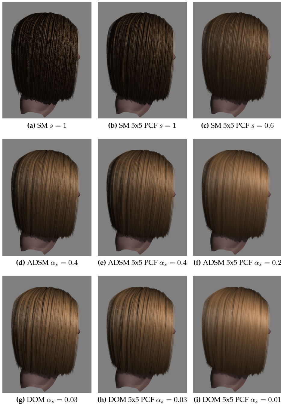
Figure 37: Comparison of SM (a-c), ADSM (d-f), and DOM (g-i). The first column shows the techniques using one sample only, whereby a 5x5 PCF filter was applied in the second column. In the third column, the shadow strength s and the shadow transparency \alpha_s have changed in order to get brighter shadows.
