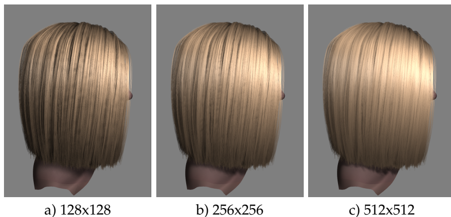
Figure 34: Shadow rendered with DOM using a opacity map resolution of either a) 128^2 , b) 256^2 , or c) 512^2 texels using a PCF kernel size of 3 \times 3 .
