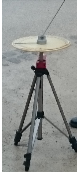
Figure 3.3: The purpose build Angular Deviation Device
