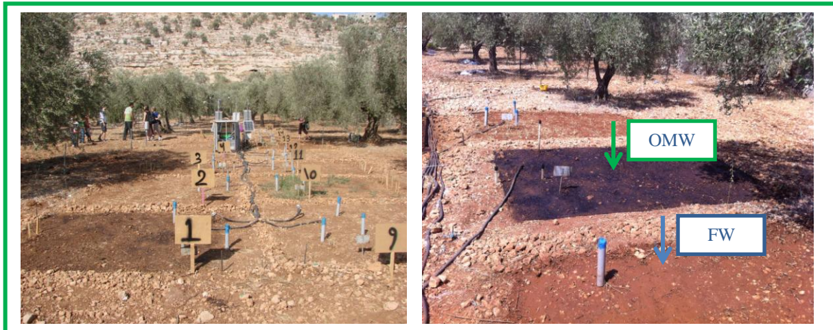
Figure 1-4: Experiment field study located in Beit Reema village-Palestine (left). An example of olive mill waste water treated plot (OMW) and control plot treated by tap water (FW) (right). (Source: Trilateral project “OLIVEOIL”, Koblenz-Landau University).
