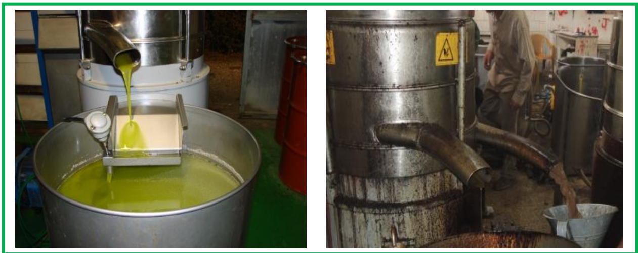
Figure 1-3: Olive oil produced by 3 phase extraction technology in Palestine (left). Olive mill wastewater produced during the oil extraction process (right). (Source: Trilateral project “OLIVEOIL”, Koblenz-Landau University).
