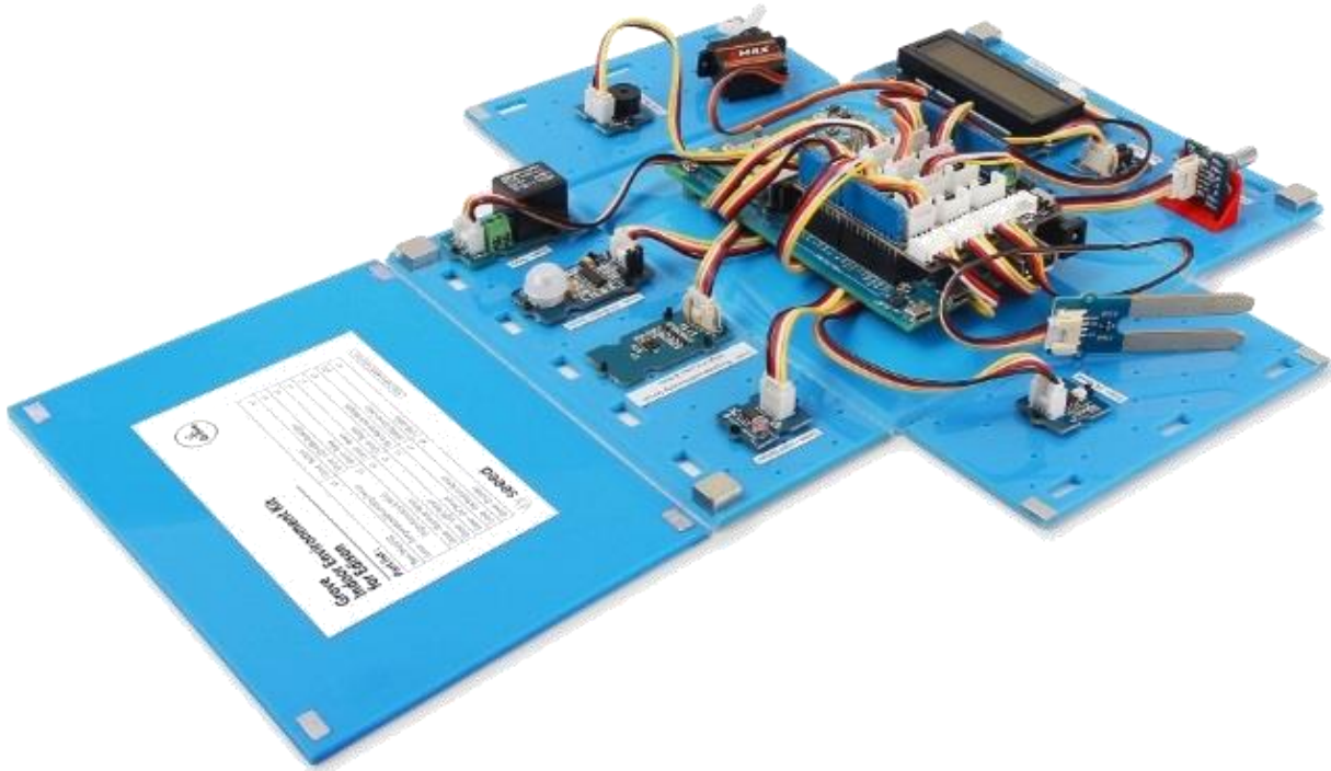
Figure 34: Grove indoor environment kit components on Intel Edison board, adapted from (Seed, 2015)
