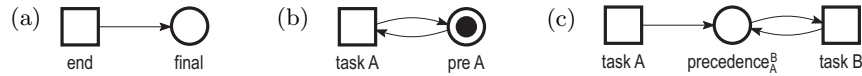
Fig. 1. The nets (a) N_{\text{end}} , (b) the building block of N(Tasks) , and (c) N(\mathbf{precedence})(A, B) .
