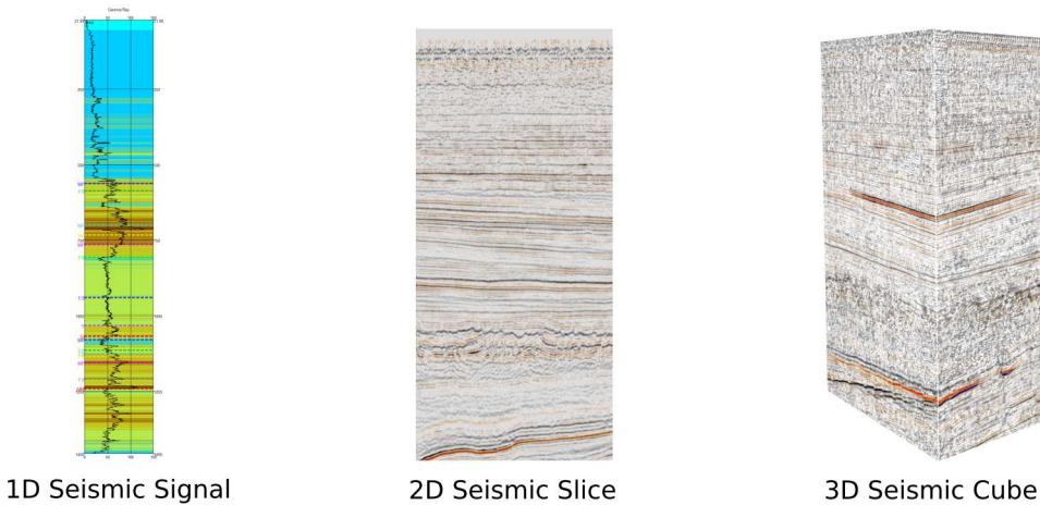
Figure 2.6: Comparison of 1D seismic signal, 2D seismic slice and a 3D seismic cube of the F3 dataset [15]
