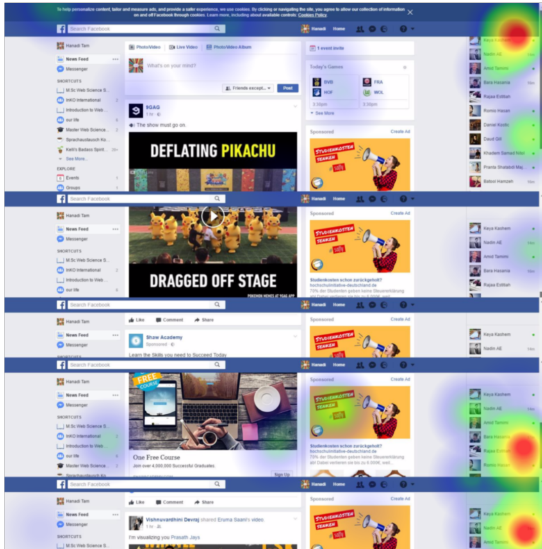
Figure 5: Illustrates the created stitched screenshot of a participant in a Facebook eye tracking study (using the Stitched-Viewport Screenshot method). Notice the replication of the fixed elements (left side navigator, sponsored ads, header, and the chat sidebar). The gaze data are scattered on each duplicated fixed element as were recorded in the session.
