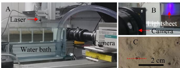
Fig. 3.3: A). Picture of the experimental setup showing the four test tanks in the temperature-controlled water bath and the \tau LIF system consisting of laser and camera. B) Illustration of the projected laser light sheet from above and the illuminated area captured by the camera. The interrogation area was 14.4 \times 19.2 \text{ mm}^2 . C) Typical burrow openings in the test tank. The image was taken in T1 before the start of the experiment. The dashed red line shows the location of the light sheet on the selected burrow opening.
