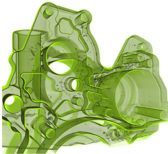
Figure 4.1: Rendering of a cast housing(667x465x512 voxels), with DVR and a two dimensional transfer function based on density/gradient magnitude. Due to the high transparency the frame rates are low, but still interactive at 3-5 frames/s on an ATI Radeon 1900XTX.
