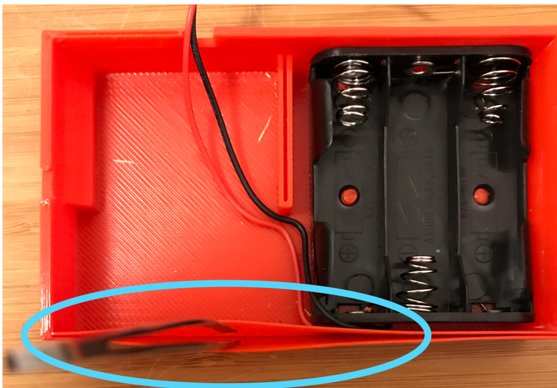
Appendix 5: Third Hardware Prototype - fragility (own illustration)
