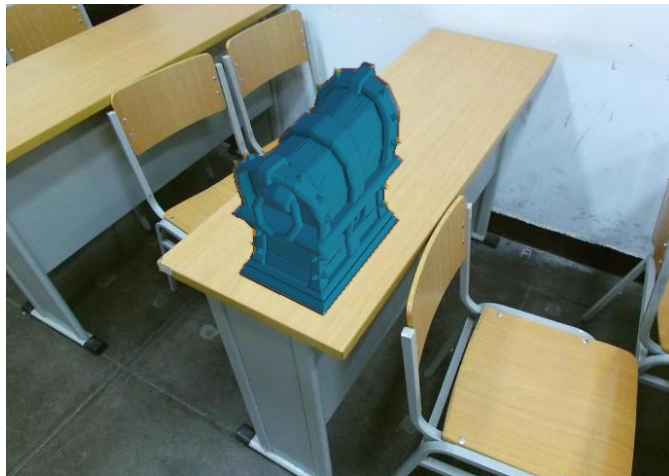
Figure 2: Mockup for the graphical output of the tracker. The tracked object is rendered on the estimated current position, which should cover the actual object in the image. The background for this image is taken from [21].
