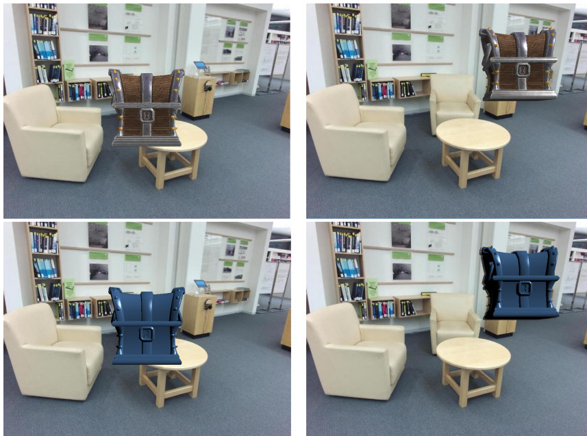
Figure 20: The upper images show the input frames, the lower ones show the object in its predicted pose rendered on top. Left side: The object in its starting position. Right side: The object was moved.
