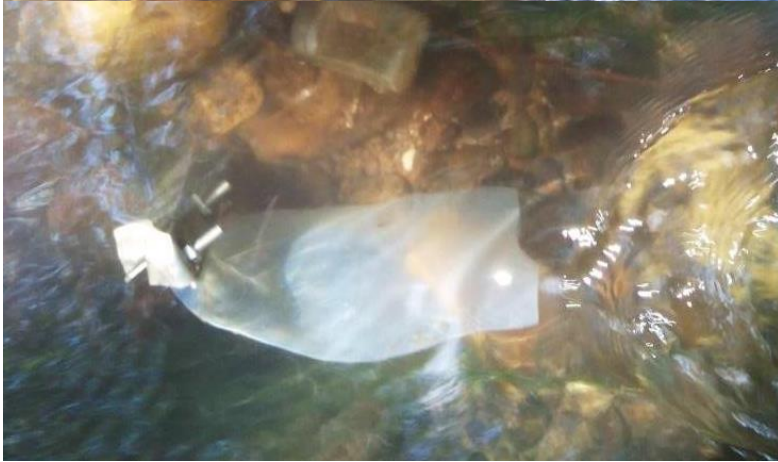
Fig. C.1: Images of passive samplers deployed in the stream. A: One replicate of Empore styrene-divinylbenzene (SDB) disk in metal holder. B: polydimethylsiloxane sheets (PDMS) sheet. Photos by Verena C. Schreiner.
