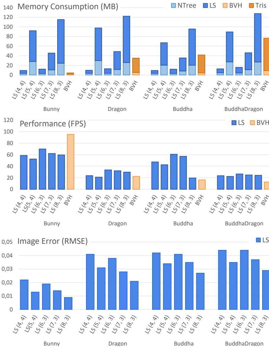
Figure 5.8: Overview of memory usage (in MB), performance (in FPS) and image errors (in RMSE) of the LS using different parameter sets and BVH for the test scenes. Using high values of N or d lead to high memory consumption but less image errors, as shown by the parameter sets of LS (5, 4) and LS (8, 3). The used memory size is nearly scene independent and mainly depends on the used parameters. The BVH size is rather small but in contrast to the LS it additionally needs the triangle information of the scene. In general, the LS results in higher performance in more complex scenes with a high number of scene triangles. Data from Table 5.1.
