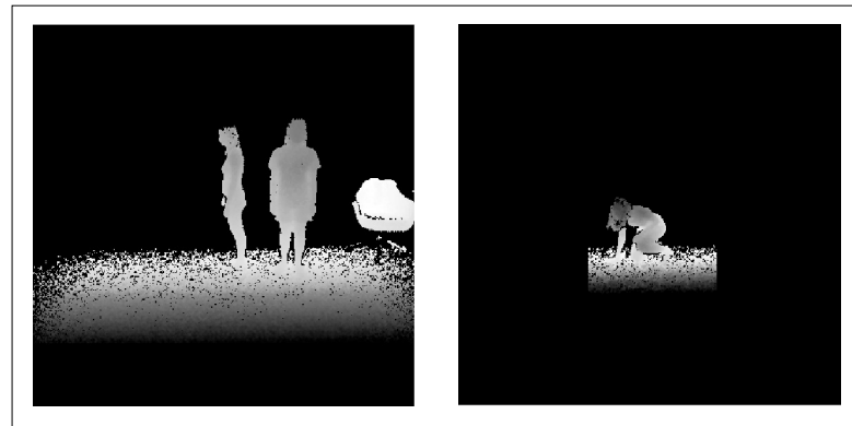
Figure 8.4: Sample frame of action from depth data. Left: Sample frame of action walking apart with noise and unnecessary object, right: Sample of action falling with overlapping of noise and body parts as well as straight cut lines in the noise area.
