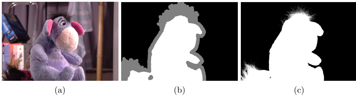
Figure 4.5: A natural image matting example. (a) Shows the input image. (b) Shows a user-specified trimap. The trimap splits the input image in three regions: definitive foreground (white), definitive background (black) and unknown (gray). (c) Shows the alpha matte. Image source: Benchmark test data set with ground truth data [RRW + 09].
