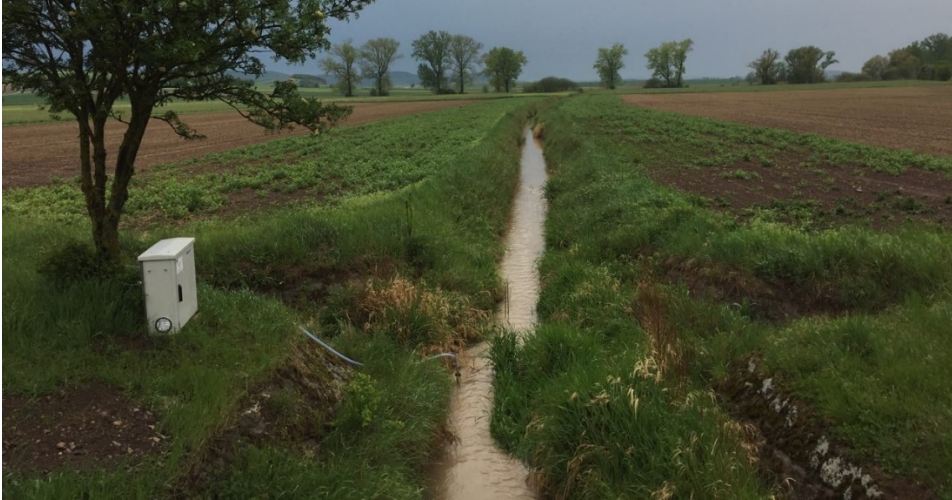
Figure 5: Automatic, water-level triggered EDS sampler installed in a typical agricultural stream to measure surface runoff-induced pesticide peak concentrations in the Kleingewässer-Monitoring (KgM).
