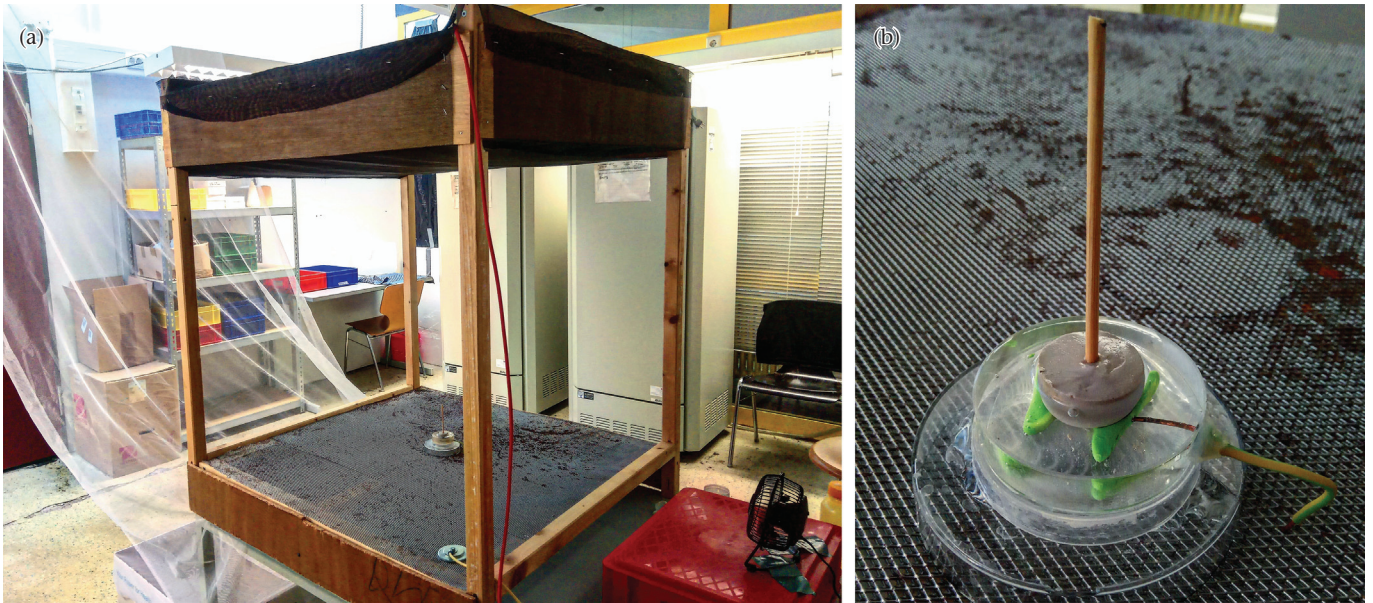
Figure A1. (a) Side view to the experimental set-up comprising the experimental frame with two interconnected and electrically grounded parallel metal electrodes, a table fan and a mesh to capture spiders. (b) Dispersal platform with a vertical stick made of moist plaster of Paris and connected to the bottom electrode via a wire.
