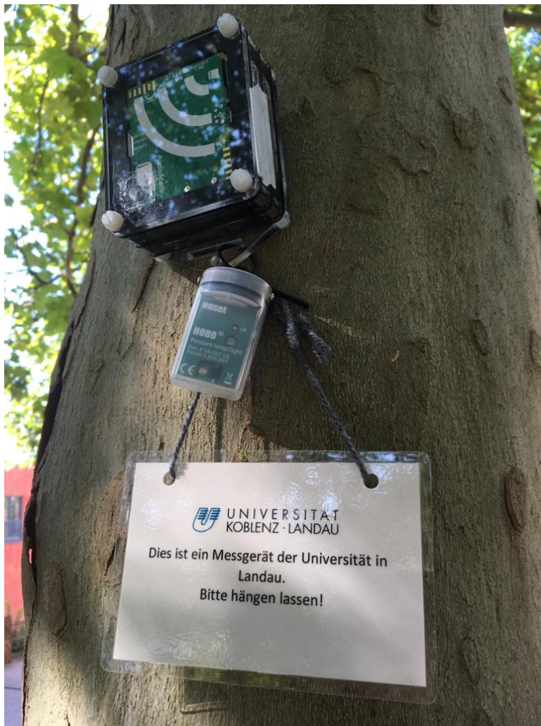
Figure 26: An AudioMoth device fixed to one of the trees with a HOBO logger hanging from it
