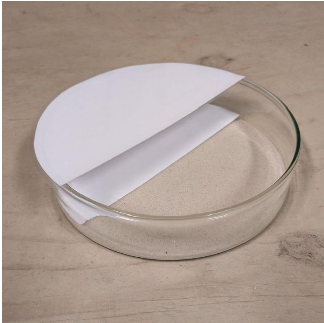
S2 Fig.: Glass petri dish filled with silica sand before the pesticide application. One side is covered with laminated paper semicircles to prevent contamination of the clean side during the application process.
