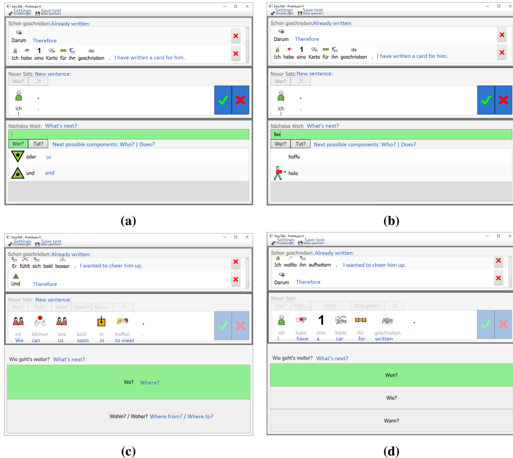
Figure 5.15: Four snapshots showing the free writing mode of EasyTalk . In (a), the default mode is shown in contrast to the free writing mode in (b). In (c) and (d), the last word added to the Sentence Panel can be assigned to different sentence components. The system presents the user with the respective options in a decision dialog.
