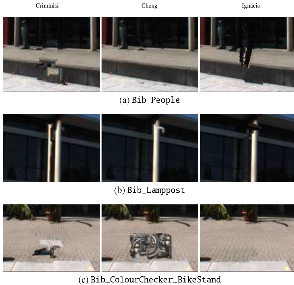
Figure 4.10: Excerpts from the inpainted images using Criminisi, Cheng and Ignácio approaches respectively.
