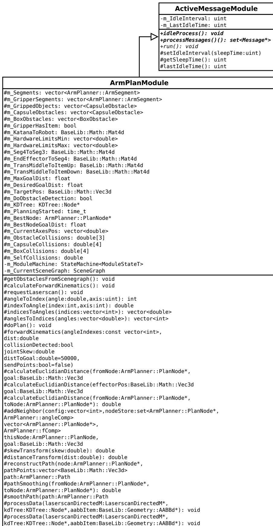
Figure 3.5: Class diagram for the path planning Module ArmPlanModule. Some member variables removed for legibility.
