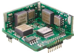
Abbildung 2.4: Inertialsensoren, Inertial Measurement Unit (IMU)
