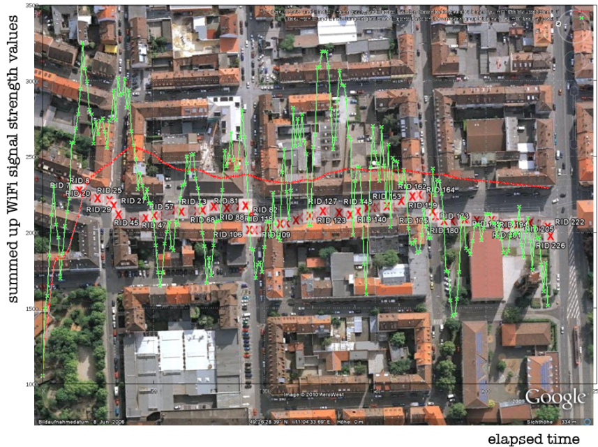
Figure 9: Overlaid WiFi measurement data from a test run along several blocks of houses
