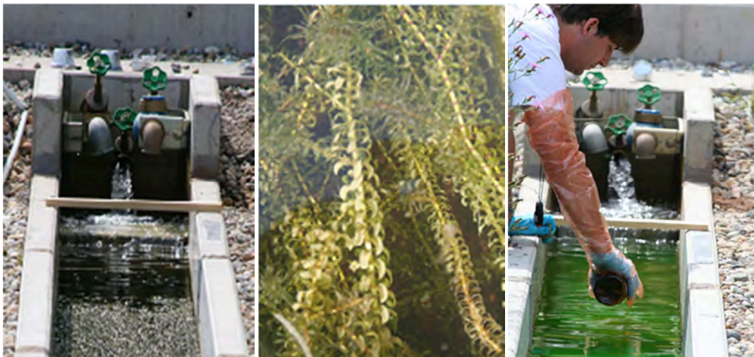
Figure 2.1.3: First picture: Inlet of a ditch. The tap on the left is for circulation of the water through pumps within one ditch, the tap in the middle provides water supply through passive feeding from the reservoir and the tap on the right is connected to communal water supply. Center: Elodea nuttallii . Right: Water sampling (Stang et al., 2009)
