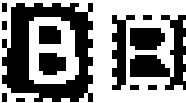
Figure 71: Classification example, highest R_{ccorr\_normed}(x, y) : 0.76 (B template)
