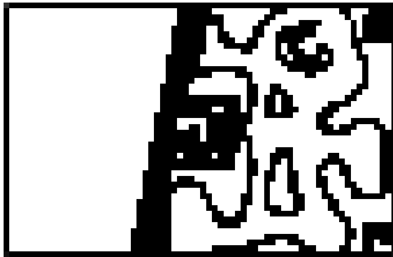
Figure 43: binary image, generated with standard adaptive thresholding algorithm (different drawing)
