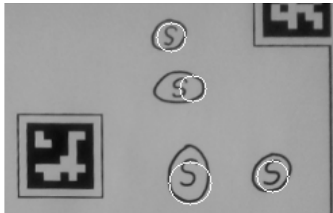
Figure 62: Test circle drawings for the S template, detected circles shown in white
