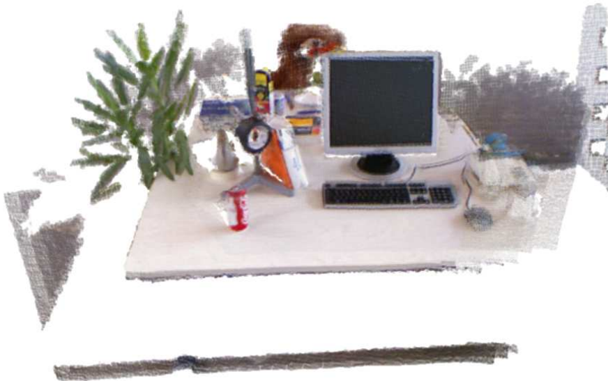
Figure 6.16: Registered point clouds using the PSO local pose estimation. The down-sampling step of the complete point cloud after each registration step leads to "layers" of points, which are visible on the outer scene areas caused by camera motion. The sensor data acquisition from different views has almost covered the invisible area behind the red can. Meanwhile, the points on the can itself are registered correctly.
