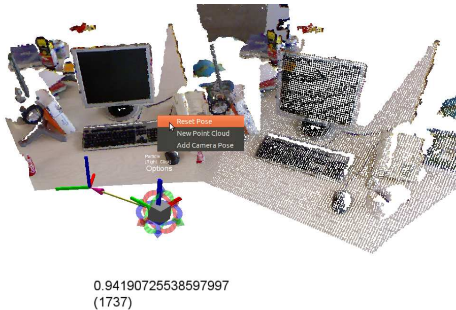
Figure 6.15: Application of an interactive particle with context menu and cost value of particle's transformation with the number of neighboring points in brackets on the bottom
