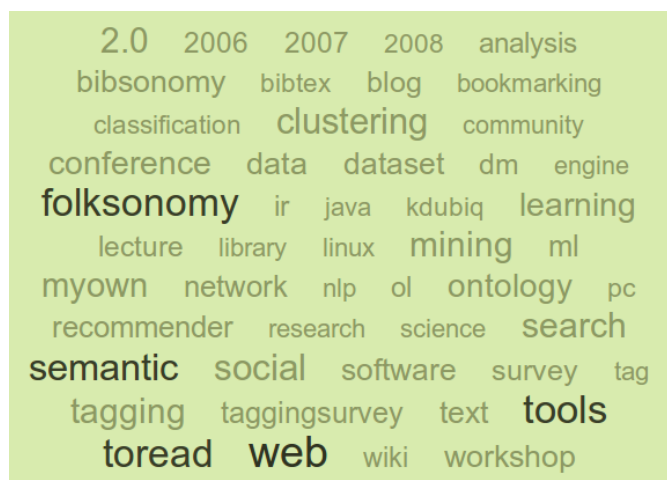
Figure 2.4: Example tag cloud from http://www.bibsonomy.org/ . The tags are ordered alphabetically. The font size and intensity indicate the frequency with which the respective tags are used in a collection of resources.
