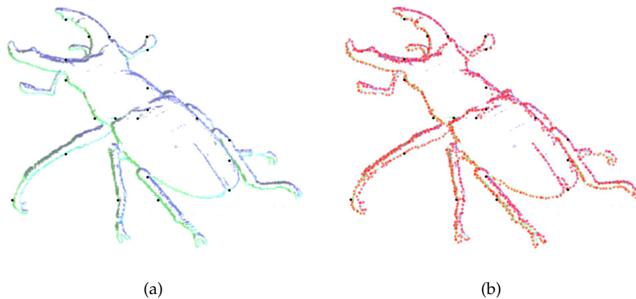
Figure 18: Contour seed points, (a) initial points as black dots and (b) points detected with line-following algorithm as red dots.
