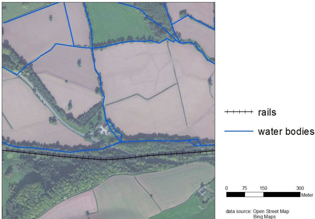
Figure 69: Example situation where a stream flows along rail for a certain length. The stream is accompanied by riparian vegetation and hardly gets closer than approximately 10 m.
