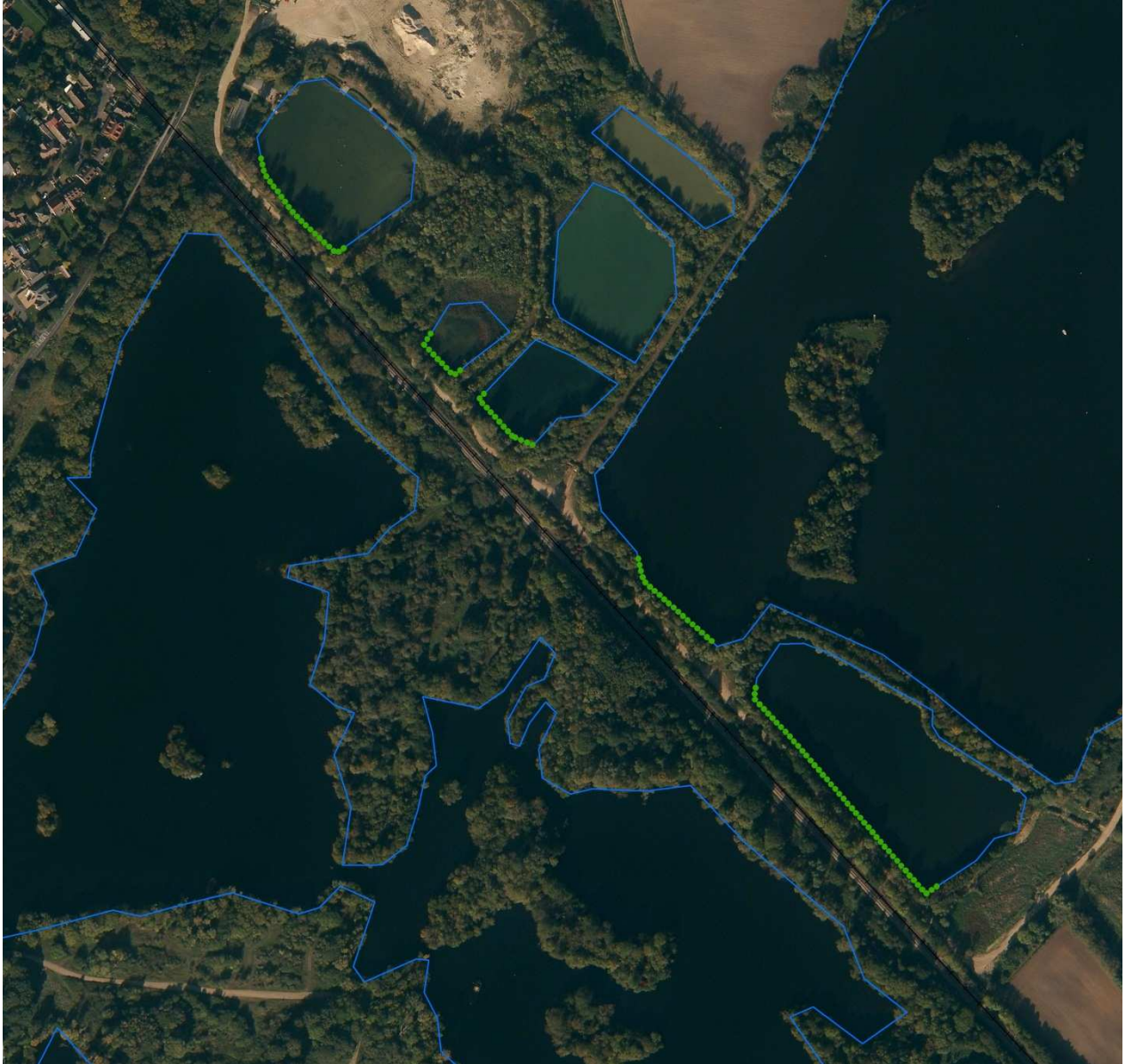
Figure 74: Spatial distribution of PEC sw for riparian water zone of ponds and small lakes (1 MC run). Railway running from north-west to south-east; western wind direction; dots indicate WB segments in \leq 50 m distance to rails; spray-drift filtering by riparian vegetation not taken into account (green dots: TER \geq 1 ). No TER = 1 violation due to considerable rail-to-WB distance.
