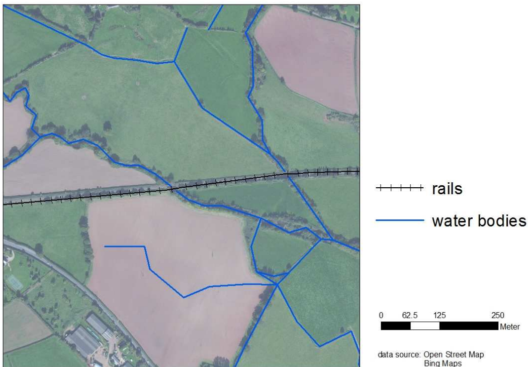
Figure 68: Typical situation where WBs cross a railway. Their fraction close to rails is therefore small. Water bodies cross railways often in pipes underneath embankments.
