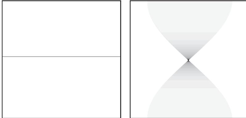
**Figure 17:** A line and its resulting Hough accumulator. Every point of the line gets mapped to a sinusoidal curve in the accumulator. The common point of intersection of all curves represents the line  $(d, \alpha)$  of the input image on the left.
