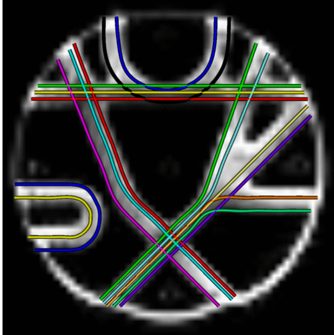
Figure 3.16: MICCAI Fiber Cup hardware phantom: The dataset imitates a coronal human brain slice and comprises challenging intra-voxel fiber configurations such as fiber crossings, kissings, and fannings.
