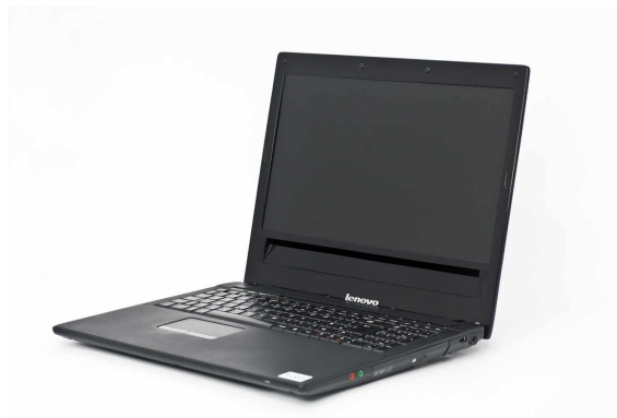
Figure 2.7: Tobii prototype of a laptop with eye tracking unit.
