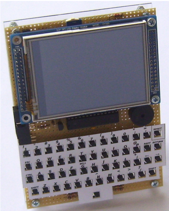
Figure 17: front image of the final (revision 3) prototype with keyboard overlay and all components.
