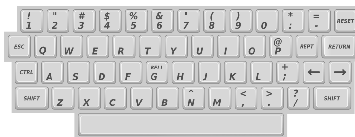
Figure 3: sketch of the Apple ][ original keyboard with all its 52 keys (the power lamp at the lower left corner not included) [21] (p. 6).
