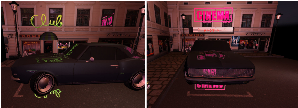
Figure. 41: Missing occlusion for the reflection on the street. The reflected ray should be blocked by the parked car.
