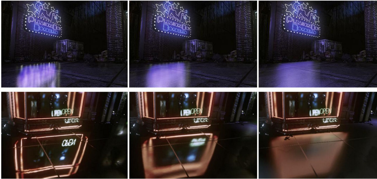
Figure. 2: Blurred reflection in Unreal Engine 3 tech demo Samaritan , top: different amounts of anisotropic blurred reflection in y -direction, bottom: different amounts of isotropic blurred reflection (images: [MD11])
