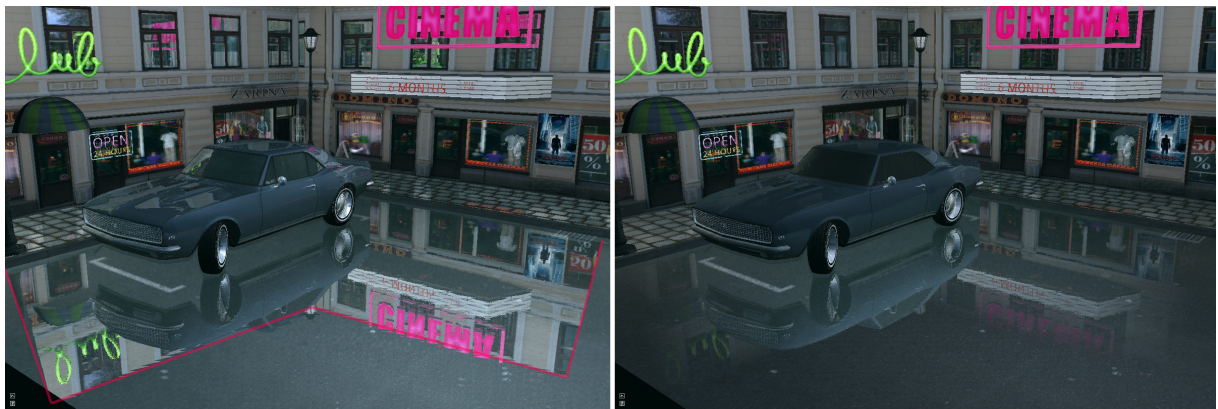
Figure. 49: Optimized SSR, Left : SSR creates clipped edges at the screen borders (marked with red line), due to the missing information originating from deferred shading, right : fading out at the screen borders creates a visually more appealing effect.
