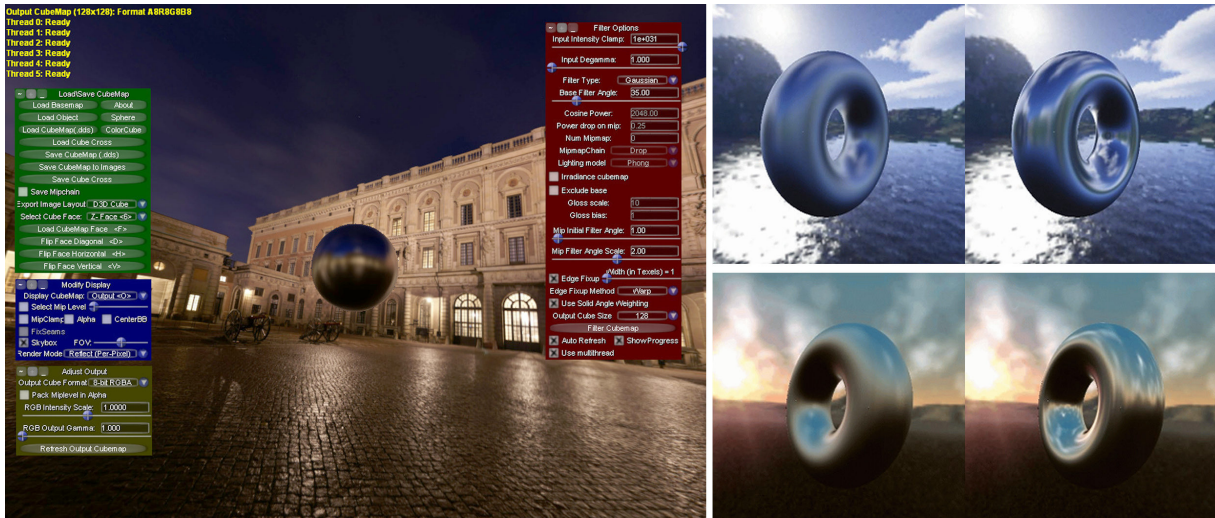
Figure 20: Left: AMD CubeMapGen generates prefiltered environment maps, right: Reflections achieved with prefiltered environment maps, right images: [KVHS00]
