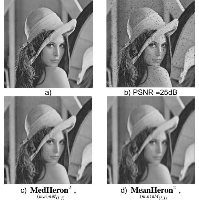
Fig. 1. Original (a) and noise (b) images. Denoised images (c) PSNR=31dB, and (d) PSNR=28dB
