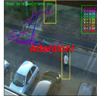
Fig. 6. The logical inference has found a possible case of a street offence in the graph of blob trajectories. All probable participants of the conflict are marked by yellow rectangles. Multicoloured lines denote tracks of the blobs. The program estimates the velocity of the blobs and depicts it by different colours. Direct blue lines depict possible links between the blobs.
