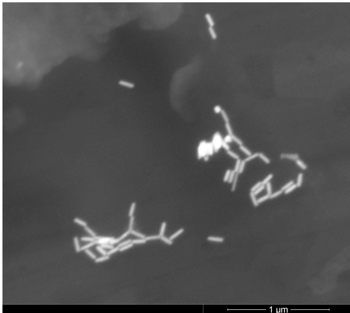
Figure S1: Representative SEM picture obtained using a back scattering electron detector of the silver pentagonal prisms (nominal length of 165 nm).
