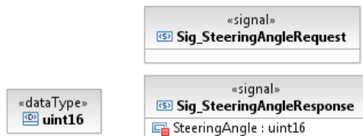
Figure 5.6: The Signals and data types corresponding to the communication scenario illustrated in Figure 5.5
