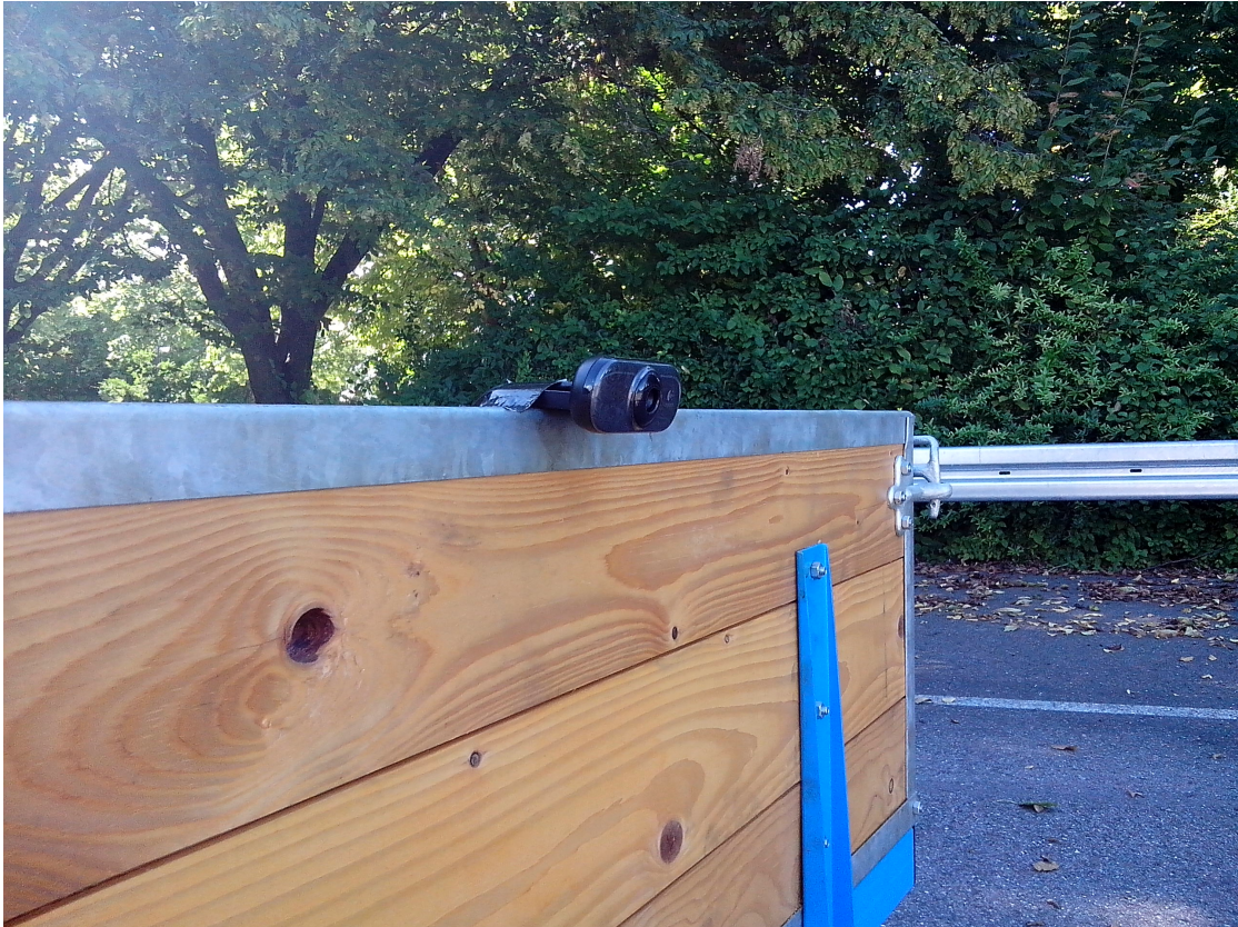
Figure 9.4: Simple USB webcam to create a picture of the area behind the trailer.
