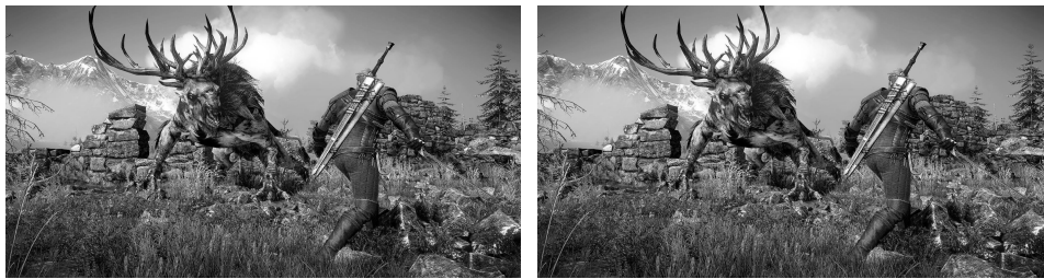
(a) Kompressionsrate: 50%; Bitrate: 15.99; MSE: 66.6; PSNR: 29.8 dB (b) Kompressionsrate: 20%; Bitrate: 6.4; MSE: 303.9; PSNR: 23.3 dB
